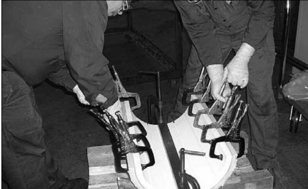
Figure 7: Clamping with slight force SXL to metal housing
