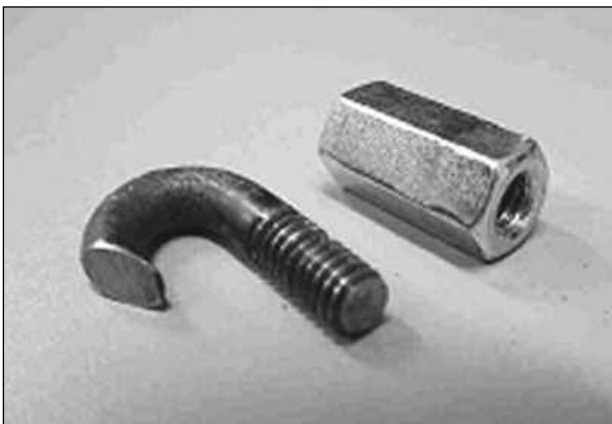
Figure 5: J-hook and nut used to remove bearing segments
